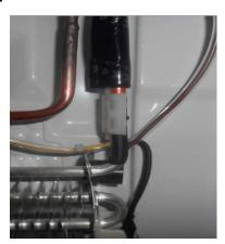
The Sensor mounted incorrectly: Facing the rear and too low.
