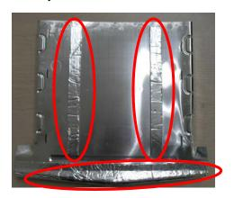
7. Bend the bottom row of the cooling ribs on the evaporator.
